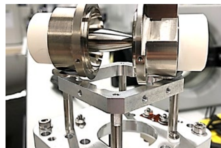
An ultra-high resolution / accurate mass spectrometry Orbitrap™ mass analyser for chemical and biomolecular analysis
