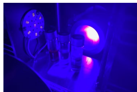
A photoredox chemical reaction illuminated by light emitting diodes. Image credit: Anastasios Polyzos, UoM.
