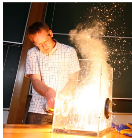
Mick performing the thermite reaction between aluminium and iron oxide.
