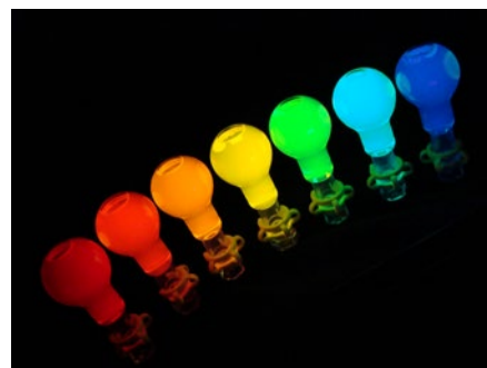
Quantum dots are small semiconductor crystals just 1-20nm across. Their size controls their optical properties. The image shows luminescence from cadmium selenide crystals, ranging in size from 1-6nm.
