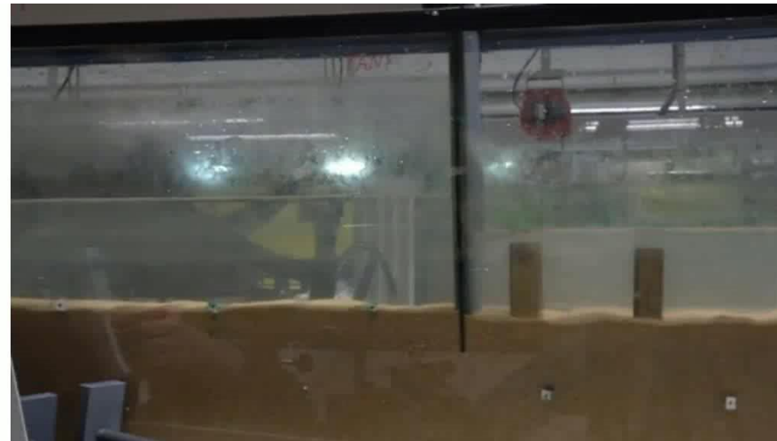
Sand boiling/quicksand condition
