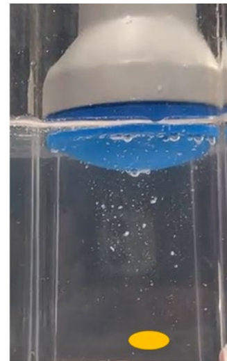
A high intensity focused ultrasound probe showing how the beam is focused at the target (oval shape) rather than fan-shaped like a diagnostic probe.
