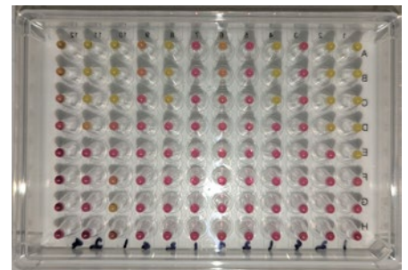
A colorimetric LAMP assay, where yellow/orange tubes indicate the presence of the target pathogen and red tubes are negative.
