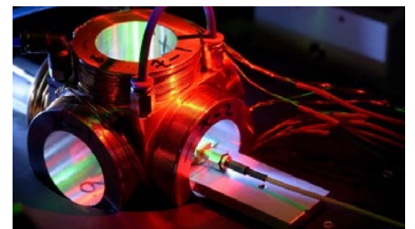
Precision sensing with a quantum-based diamond magnetometer.
