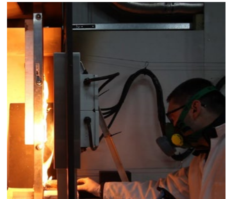
Testing fire resistance of facade materials.
