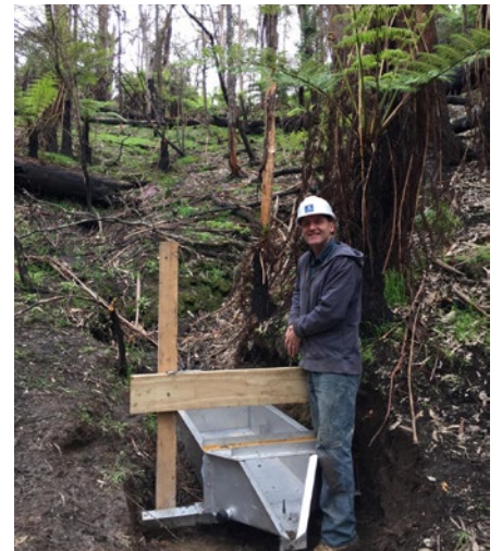
Installing runoff monitoring equipment on hillslopes after a bushfire.
