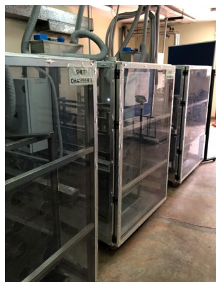
Methane chambers at ILRI, Nairobi measuring from Boran cattle and Red Maasai sheep.
