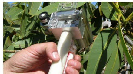
Measurement of tree transpiration on a dwarf eucalypt using a porometer.
