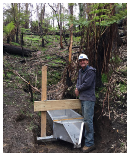
Installing runoff monitoring equipment on hillslopes after a bushfire.
