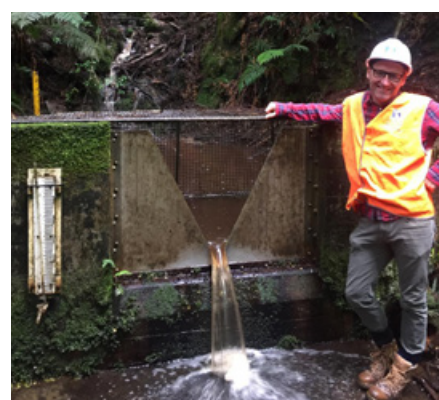
Using “instrumented catchments” to understand how rainfall, forests, and runoff interact.
