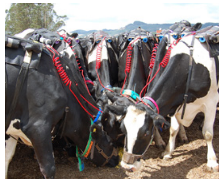
Methane being measured from Dairy cows using the SF6 technique.
