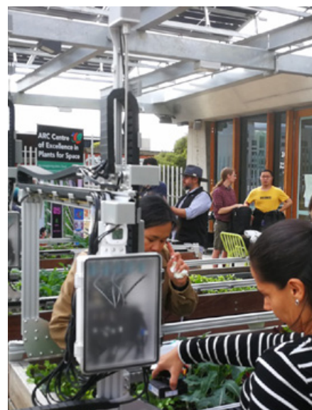
Robotic farming systems in Parkville to produce pick-and-eat leaf vegetables implementing digital sensors, AI and digital twins.
