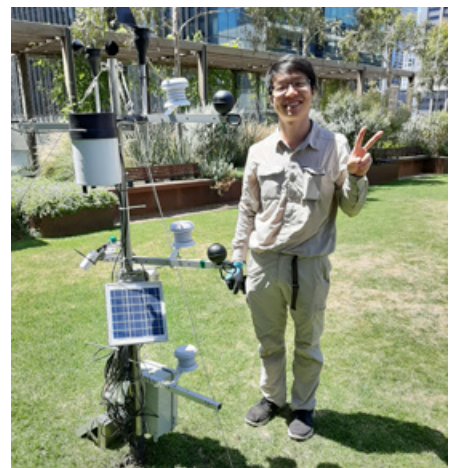
Measuring the microclimate and energy balance on a green roof in Docklands, Melbourne.
