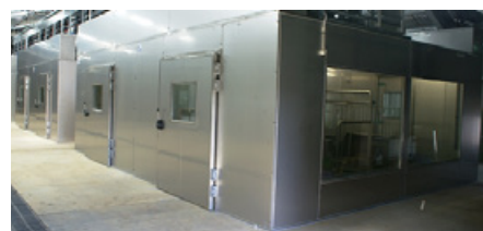
Respiration chambers for measuring enteric methane
