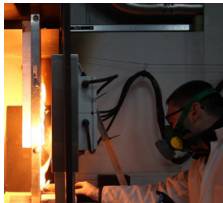
Testing fire resistance of facade materials.
