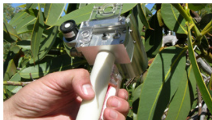
Measurement of tree transpiration on a dwarf eucalypt using a porometer.
