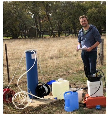
Sampling groundwater from a well bore for water quality analysis.
