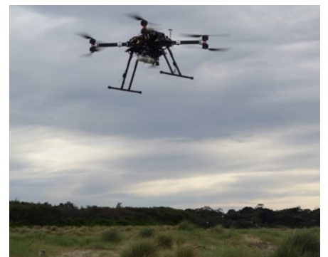
Drone-based aerial laser (LiDAR) surveying of beach change in Victoria to enhance coastal resilience to climate change.
