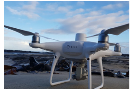
A Phantom 4 RTK drone used for citizen-science surveying as part of the Eureka Award winning Victorian Coastal Monitoring Program.
